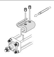
• The above figure shows the mounting example of the D-A9 $\square$ (V)/M9 $\square$ (V)/M9 $\square$ W(V)/M9 $\square$ A(V)L.
