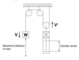
3. The following selection example and procedures are based on use at the intermediate stop (including emergency stops during the operation). However, when the cylinder is in the locked state such as drop prevention, kinetic energy does not act upon it. Under these conditions, use the load weight at the maximum speed (V) of 100 mm/s shown in Chart (5) to (7) on page 2 depending on the operating pressure and select models.
