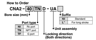
\* The lock unit for long stroke is applicable only to the flange style with 1001 stroke or longer whose bore size is ø50 to ø100. (Example: CNA2-100D-UAL)
