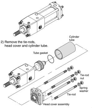
Apply 44 psi or more of compressed air to the unlocking port, and pull out the piston rod assembly.
