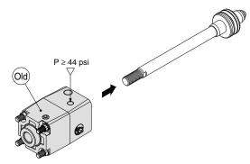
4) Similarly, apply 44 psi or more of compressed air to the unlocking port of the new lock unit, and replace the new lock unit's temporary axis with the previous piston rod assembly.
